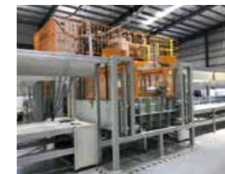
Helium inspection line
